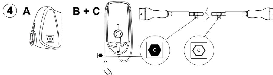
EN This label and its indicated location on the charging station are in accordance with Directive 2014/94/EU (Alternative Fuel Infrastructure Directive) and EN 17186. The charging station owner is responsible for applying the label. Local laws and regulations must also be obeyed. See fuel-identifiers.eu for more information.
